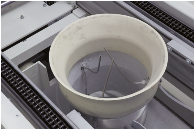
Patented docking collar with cleaning device
