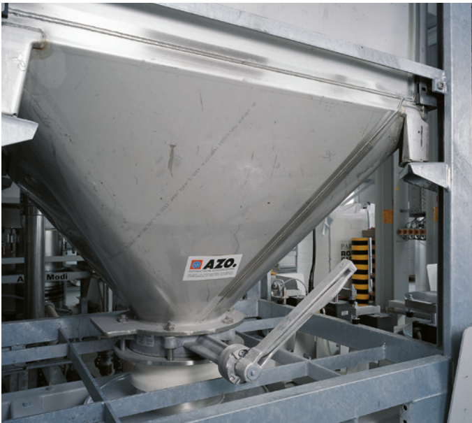
The patented docking collar establishes a dust-free connection between the flap-type outlet of the container (or bin) and the downstream inlet piece.
