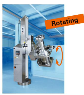
With the new Lifting column it is possible to rotate packing drums and empty them after docking with hoppers or processing equipment.
