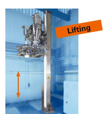
Up to 6 different positions can be assumed for the various working steps, e.g. loading at floor level, several working positions, servicing.
