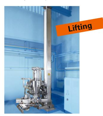
The Lifting column accepts drums or corresponding modules at floor level and raises them to the required working position.
