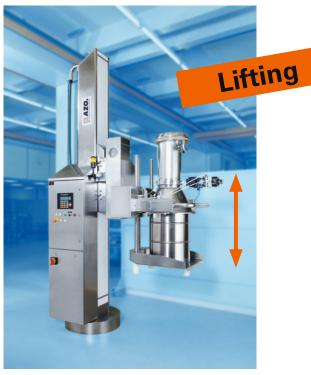
A freely programmable controller lifts modules or docked drums accurate to the millimetre.
