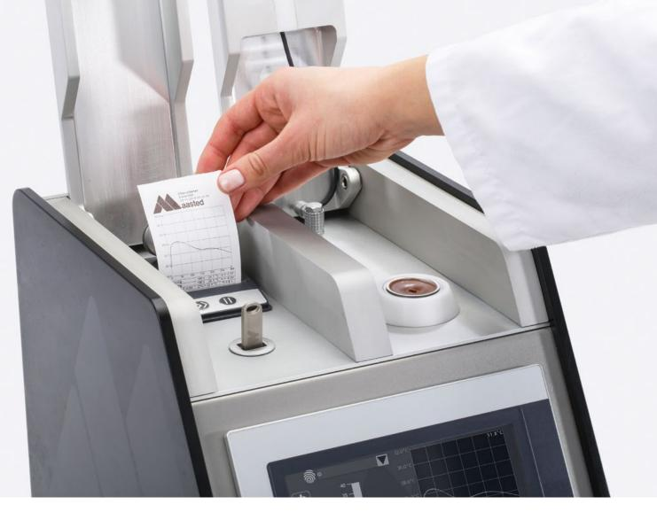
Chocometer+ calculates the CTU (Chocolate Temper Unit) and the slope. It also computes and displays the Temper Index (TI).
