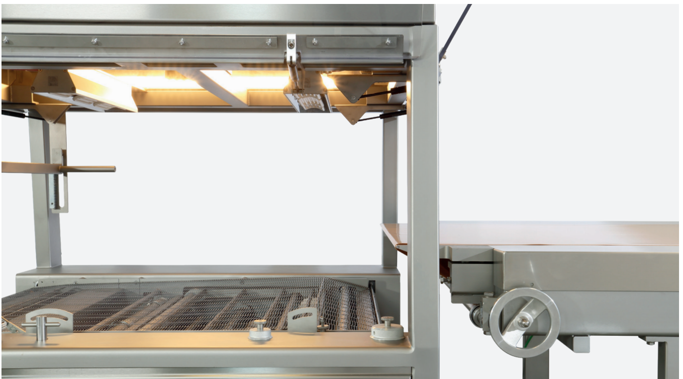
The bypass solution enables you to easily have a conveyor belt going through the enrober.
