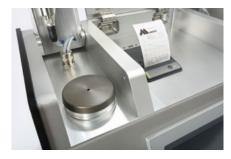
The sample reactor within the ChocoAnalyzer instrument.
