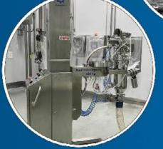
Vacuum Transfer System installed on Mobile Lifting Column
