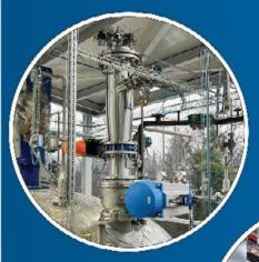
VTS model AGR400 for reactor loadina at a height of 10 meters with a capacity of 800 kg/h.
