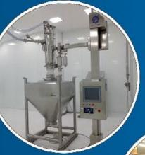
Vacuum Conveyor to load a Roller Compactor
