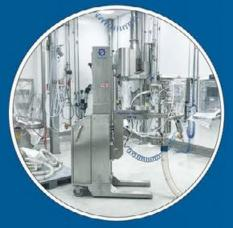
Automatic Mobile Lifting Column for Vacuum Conveyor
