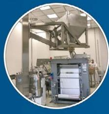
Bin Lifting Column connected to the sachet packaging machine
