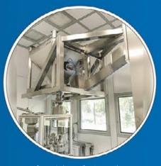
Lifting Column for Bin with an integrated vibration system
