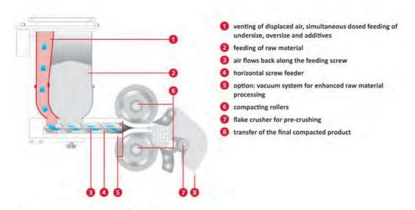
Optimized feed through the Combi-Vent-Feeder® technology illustrated on the example of a WP 200 Pharma
