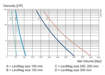
Figure 5. Duty Level 3: Mixing Volume vs. Vicosity
