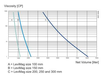
Figure 4. Duty Level 2: Mild blending Volume vs. Vicosity
