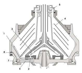
Typical bowl drawing for a vortex nozzle centrifuge. Drawing details do not necessarily correspond to the centrifuge described.
