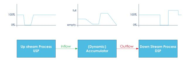
Typical characteristics of discontinues processes balanced out by a Dynamic Accumulator.
