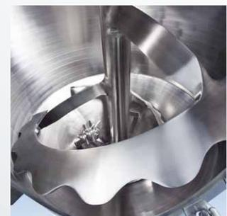
SinConvex® mixing tool for up to 99,99% complete discharge
