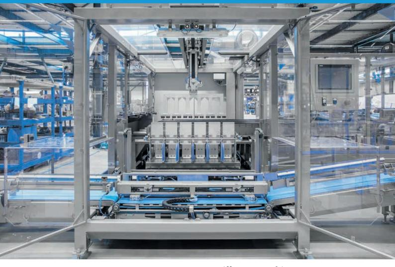
The Gantry series offer a wide range of solutions for many different horizontal or vertical packing applications. These solutions are designed for case packing of large quantities of bags coming from single or multiple bag makers. They put individual packages into trays, cartons or other secondary containers. These innovative systems from BPA outperform conventional solutions.
