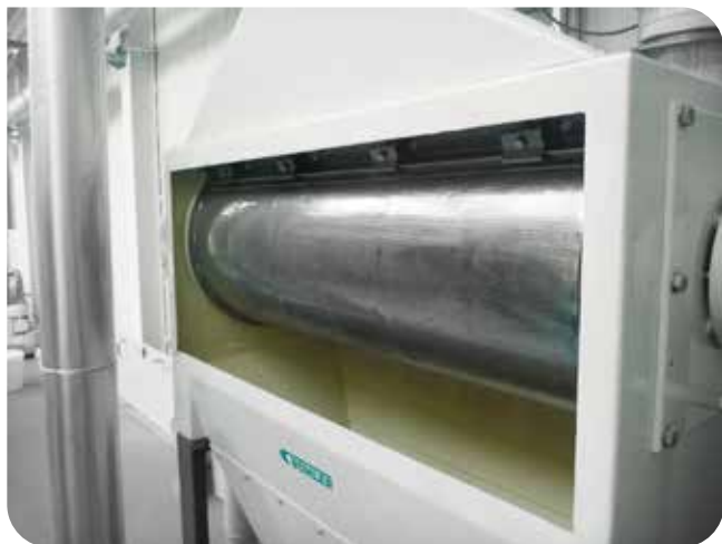
Maximum yield thanks to efficient separation of flour particles adhering to the bran.
