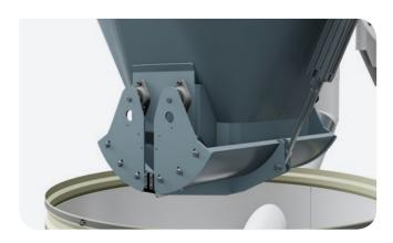
Double segment slide gates made from stainless steel with high wear resistance.
