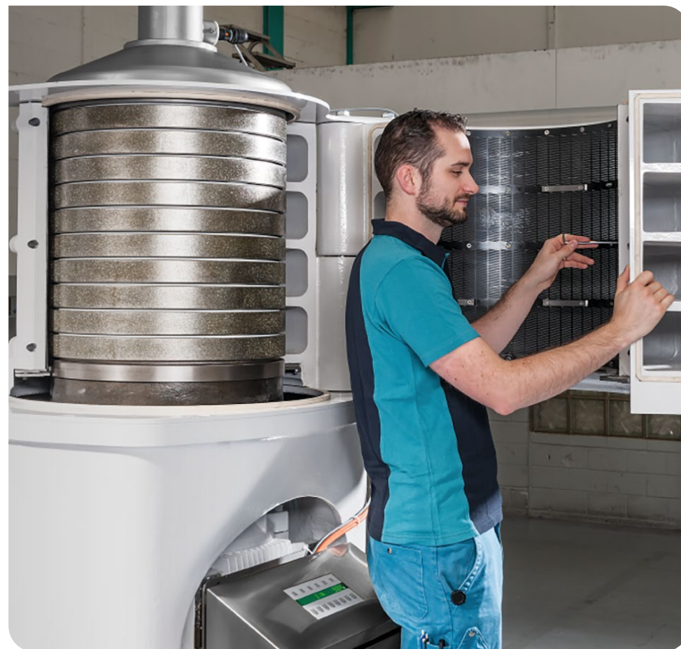
Osiris – maintenance-friendly thanks to a fold-up air channel
