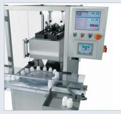
With the TC 8210 Tare-Gross each container is weighed before and after filling. The actual content is measured with high accuracy and weight deviations of the containers are eliminated. In conjunction with a counting machine, the combination of two different systems (counting and weighing) provides the maximum certainty to exclude an error.
