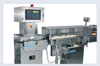
For the use in extremely rough environmental conditions (e.g. wet rooms) we offer the water jet proof checkweigher TC 8500. In the tinned food industry this type has produced an output of up to 450 weighings per minute for many years. The whole machine is washable with high water pressure.
