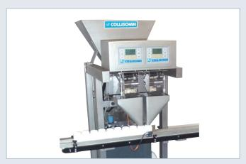
Twin Weigh filler \$ 706-2 with automatic filling station for higher output. On demand the machine can be equipped with many weighing heads.
