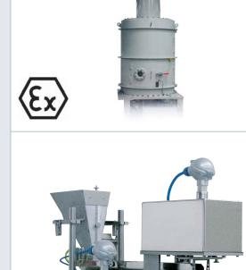
The weigh filler Ex 703 doses explosives in airbag inflators. It can be delivered with an explosion proof enclosure.
