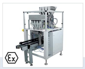
Ex 706-4: The multiple linear weigh filler doses explosives of 30.000 mg with an accuracy of  $\pm$  3 mg at a speed of approx. 25 weighings per minute.
