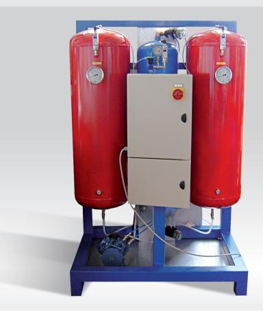
The system collects potentially radioactive air from inside hot cells during radiopharmaceutical production or after a malfunction of the synthesis modules.
