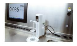
**Dose calibrator\*** - The ionisation chamber compartment is at the centre of the machine work surface. The sample holder lifter automates the lifting action of the vials/syringes from the ionisation chamber to the work surface and vice-versa.
