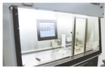
Work chamber - Spacious work chamber made of AISI 304 stainless steel for maximum ergonomics, equipped with a motorised safety 8 mm thick glass window. A 17" monitor integrated in the rear side of the work area, used to control the dose calibrator\*.
