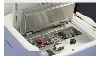
Safe and easy positioning of the disposable main kit. Compatible with different types of shielded containers for vials (see our technical datasheet for more details).
