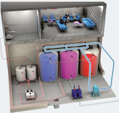
5) **Automatic collecting and measuring unit:** the system measures the sample obtained from each decay tank.
