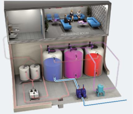
6) **Discharge unit:** after sample measurement, if the activity and concentration levels are below preset values, the examined tank can be discharged by pressing the appropriate button on the control panel.
