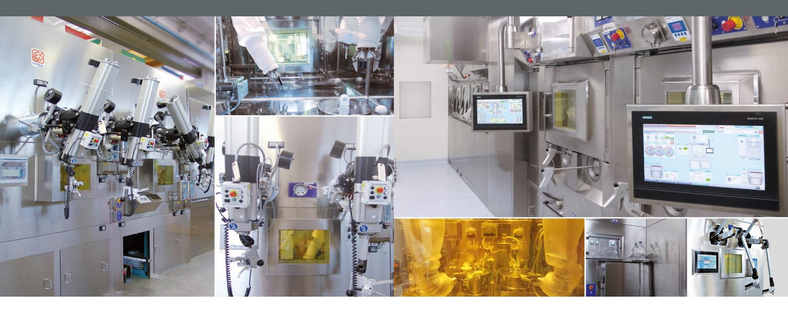
Production plant consisting of two high-shielding hot cells in which it is possible to perform fractionation, calibration and preparation operations for shipment of 99Mo bulk.
