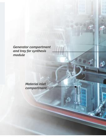
The new shielded THECLA isolator with an integrated dispensing system for radiopharmaceuticals consists of:
