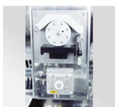
The main chamber is fitted with a fractionator system of radiopharmaceuticals in single-dose syringes of both PET/SPECT isotopes and RADIOMETABOLIC THERAPY.
