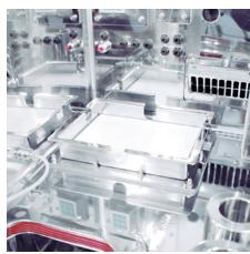
The cell is equipped with a compartment suited to house a 68Ge/68Ga generator.
