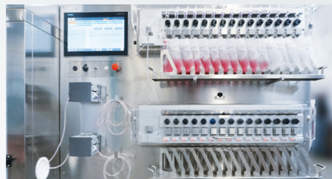
The filling rack portion with bags, bubble sensors and pinch valves
