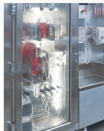
The refrigeration module contains multiple paddle mixers for gentle squeezing of source bags, ensuring a homogeneous mixture
