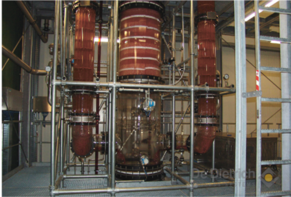
QVF type 2 shell and tube heat exchanger with SiC tubes for the condensation of distillates containing chloric or sulfuric acid.
