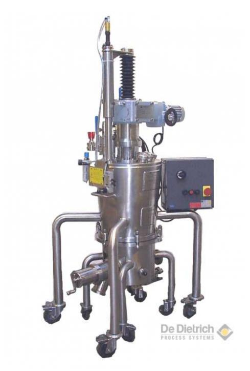
RoLab allows users to carry out all steps of a professional modern filtration and drying procedure under cGMP and FDA guidelines. The installation enables fast and frequent product
