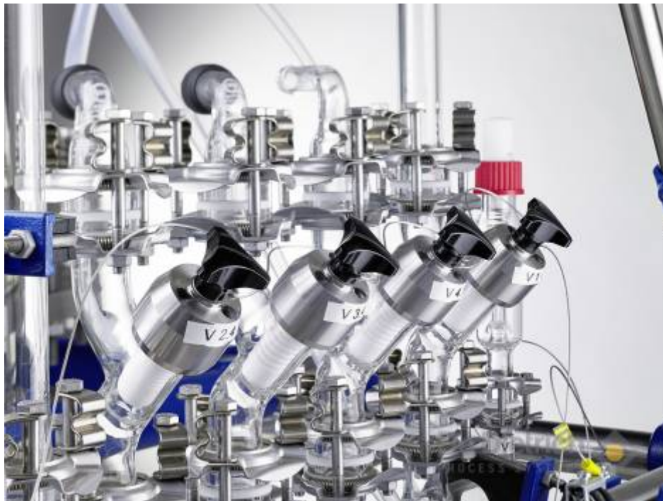
Valve arrangement of the vacuum connection
