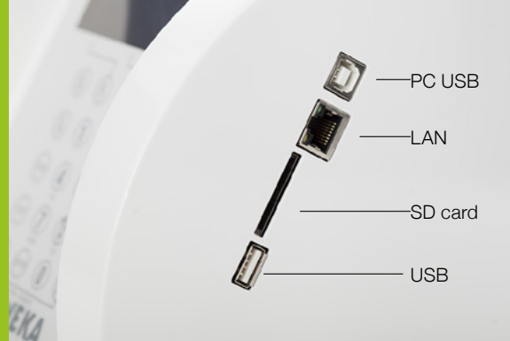
Versatile interface (USB, LAN and SD card)
