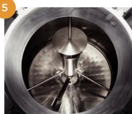
**Vigorous boiling system with internal tubular heater.**
