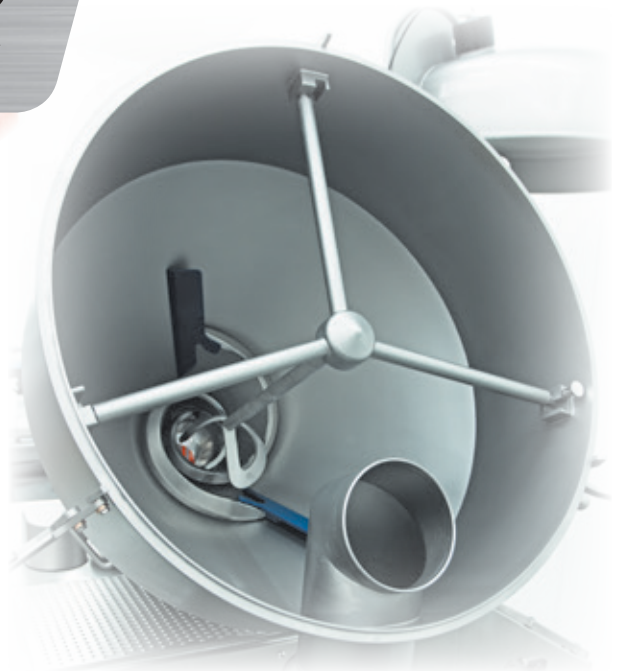
Filling hopper with double stirrer, feeder screw and feed opening for vacuum loading
