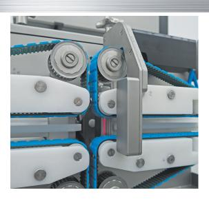
Drive of the belts with servo-motor Higher belt-speed and higher dynamic.
