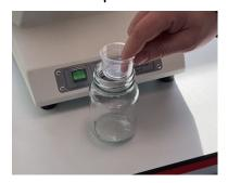
The sample container for small quantities up to 32 ml are used for 1:10 and 1:8 sample division. The 32 ml sample containers are inserted into the sample vials. The 250 ml and 500 ml sample vials can then be inserted into the divider head as described in  $\leftarrow$  Chapter 6.1.1 'Screwing the glass laboratory bottles onto the 1:8 or 1:10 dividing head' on page 17.
