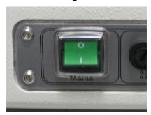
Switch main switch to I. The rotary cone sample divider starts up.
