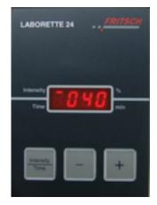
You can switch between the feed rate and timer function settings with the Intensity/Time key. Press the Intensity/Time key repeatedly until the light bar indicates the word Intensity.
