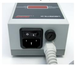
Actuate the main switch on the rear of the device. The parameters set last are displayed.
