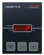
You can switch between the feed rate and timer function settings with the Intensity/Time key. Press the Intensity/Time key until the light bar indicates the word Time.
