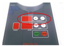
The vibration frequency can be set as 15-50 Hz (strokes per second) in 1 Hz steps using the  $\pm$ -buttons (oscillation). The mill generates natural oscillation of higher or lower intensity depending on the stroke frequency. The set oscillation frequency is controlled by the microprocessor and thus guarantees reproducible grinding.
