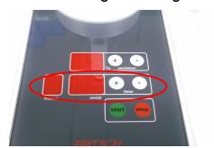
The running time is set using the +/- buttons (timer). In the factory set mode, the two right-hand numbers show the minutes and the left-hand number the hours. 9 hours 59 minutes is the maximum time which can be set. For grinding operations that are accurate to the second use the minutes/seconds timer (see → Chapter 4.6 'Changing the timer' on page 17).
