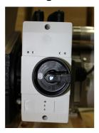
Set the main switch to ON (I). The Cutting mill starts running.
