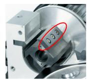
**4.** The fastening screws of the rotating knives can be unscrewed with a 6 mm Allen wrench.
