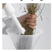
The plunger has two different sides for feeding the sample material in the funnel for long and bulk solids into the grinding chamber. On the one hand, the smooth, round side is suitable for finer material. On the other hand, the cross-shaped, thinner side is suitable for long, fibrous material, such as straw.
