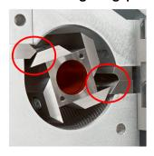
The rotating knives must not touch the fixed knives. A cutting gap of 0.2 - 0.3 mm has been set between them at the factory.
