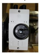
A motor protection switch turns the device off if there is an overload. (The rotary switch returns to "0").
