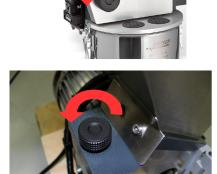
**3.** Unscrew the screw in order to open the upper half of the housing to the right side.
