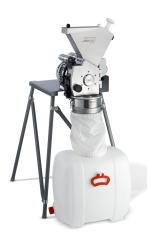
Using a fabric filter hose between the PULVERISETTE 15 and the collecting vessel allows the air flow created by the rotating rotor to be exhausted and prevents a backup. Furthermore, it accelerates the material throughput and guarantees a gentle comminution process.
