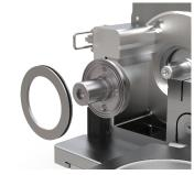
7. Clean the labyrinth seal and the seal of the cover plate.
