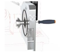
If you cannot remove the labyrinth seal just by pressing, close the closing lid with the sieve cassette inserted, but without the rotor. Take the hexagon socket screw key as described in the previous step and knock against it lightly with a hammer. The labyrinth seal should fall inwards onto the sieve cassette.
