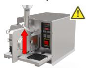
■ The closing lid (3) can be lifted out of the hinges. When opening the upper part of the housing (1), it is possible to leave the closing lid (3) in the hinge. If this is the case, make sure that the closing lid (3) does not lift out of the hinge when opening the upper part of the housing (1).
