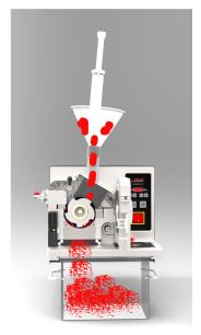
The material is fed through a funnel (example in image with standard funnel) into the cutting chamber. There, rotating knives (10) in combination with fixed knives (2,4,12) cut the material. The fine ground material falls through a sieve cassette (9) into the collecting vessel (5).
