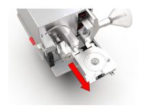
3. Clean the cone-shaped rotor holders (10).
