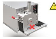
■ After checking if the rotor (10) is turning freely ( Chapter 6.1.7 'Checking if the rotor is turning freely' on page 35), the required hexagon socket screw key has to be removed immediately.
