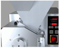
The funnel for bulk solids is fastened with four M6x12 cylinder head screws.
