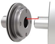
**8.** To mount the tool holder with labyrinth seal, position the cover plate on the labyrinth seal and place the tool holder with seal on the motor shaft.
