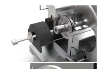
**9.** Take the anti-twist device and the M8x130 screw with the washer and mount it as shown in the picture.
