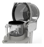
Place the silicon lid on the grinding vessel. Make sure that the lid fits properly all around.
