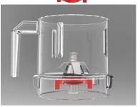
To install the cutting tool, place the knife with seal in the grinding vessel from above, and counter it from below with the bayonet lock. Make sure you insert the lock properly into the two guides. Clamp the cutting tool by turning the lock anti-clockwise (seen from above).
