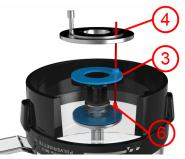
4. Insert the seal (3) and the lower bearing (4). Make sure that the holes are pushed over each other on the glass pin (6) and do not slip away.
