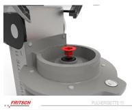
A red knife coupling (item no. 11.3205.16) is used to minimise wear on the knife holder. This knife coupling should be checked depending on the application of the PULVERISETTE 11 and whenever changing the knife. Replace the coupling with the included black spare in case of visible wear. This only serves as an emergency coupling until a new red blade coupling is available and can be installed.
