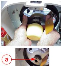
The pestle is held in place with a catch holder and can be easily removed without tools.
