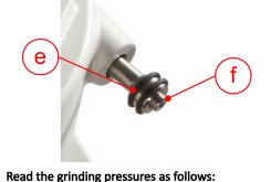
It is positioned radially in relation to the main rotation of the mortar. The desired contact pressure is built up by turning the adjusting screw (e). To do so, turn the screw (e) to the right until the display cylinder is visible (f). The contact pressure can be read on the display cylinder (f). For most applications, the lateral contact pressure is set so that the 1st ring or the 2nd ring is visible.
