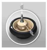
As with a hand mortar and pestle, the grinding stock is ground in the laboratory mortar mill under the influence of pressure and friction. Unlike the hand mortar and pestle, the mortar of the laboratory mortar mill is driven - the pestle axis is mounted on a rotating bearing and can be shifted horizontally. The relatively large pestle ensures fast and consistent grinding and crushing of sample material.
