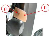
The fastener (g) of the scraper should not be tightened too firmly so that the scraper can be moved around the Philips screw (g).
