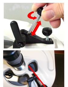
4. Move the scraper against the wall and onto the bottom of the mortar by turning it to the left.
