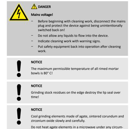
Do not heat agate elements in a microwave under any circumstances (heating is too fast).
