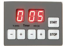
After starting the device (main switch on the back of the device), the timer shows the time setting of the preceding grinding process.
