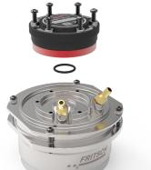
3. Lift the measuring/transmission unit (9) off of the lid (11).
