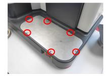
Remove the layer of rubber on the work surface and loosen the 6 screws with which the plate is attached to the housing.
