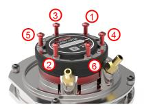
3. Tighten the hexagon screws crosswise with a torque spanner (1) until it disengages! To be on the safe side, re-tighten all screws again after initially tightening them. All screws are secured against becoming loose during the grinding process once they have been tightened with the torque spanner as described.
