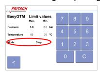
You can use the 'Mode' menu item to select how the PULVERISETTE 5 premium line is to respond to the temperature or pressure limit being reached.
