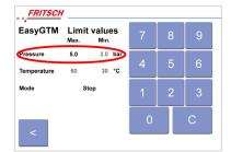
Click on the Max. and Min. fields in the 'Pressure' section and enter the maximum and minimum pressure. If the minimum pressure (14 bar) is reached, the devices goes into cooling mode or stops until the pressure falls below the minimum pressure limit. Once the minimum pressure limit has been reached, grinding continues as normal.
