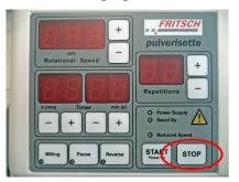
**1.** When the device has been switched off, press and hold the STOP button on the front control panel.
