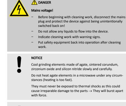
When cleaning any part of the device, adhere to the guidelines of the Accident Prevention Regulation (BGV A3) - especially if the device has been set up in a dusty environment or if processing grinding stock that produces dust.
