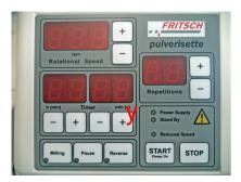
**4.** To perform changes, press the right "+" button (y) in the TIMER field: Time unit, hours and minutes  $\rightarrow$  display: -
