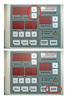
**4.** Use the +/- ROTATIONAL SPEED buttons to adjust the level of the mains voltage (90-260 V) for the existing mains system.
