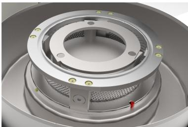
4. Place the cutting rotor on the motor shaft.
