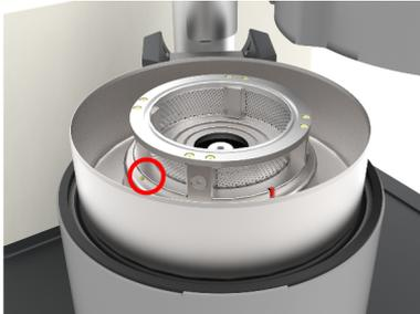
3. Position the collecting vessel while also observing the grooves and notches on the sieve support.
