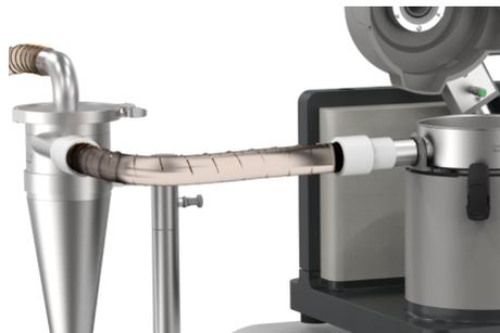
1. Slide the bushing with the spiral hose from the cyclone separator over the outlet of the grinding vessel.
