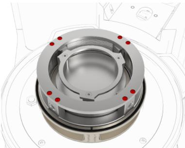
2. → Check that the fixed knives can be moved in the spring suspension. If the knives cannot be moved, loosen the 8 screws further.
