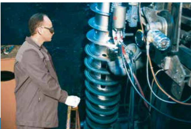
GEA tackles problems posed by abrasive particles with special armourplating for all decanter components which are at risk.
