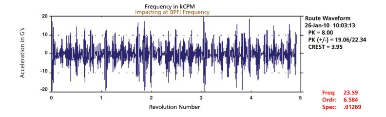
This illustration indicates a defect in the male rotor bearing (C1). Vibration analysis detected the problem, avoiding a catastrophic compressor failure.
