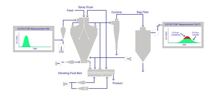
The majority of fires in spray dryers are caused when glowing hot powder lumps form and fall into the lower chamber of the spray dryer, where they can break apart and act as an ignition source for explosive dust-air mixes. These heated powder deposits release CO, which can be evaluated indirectly by using a calculation based on measurements of the amount of CO in air that enters the plant via air inlets, and the amount of CO in air that leaves the plant via air outlets.
