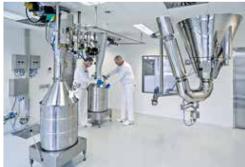
Powder collection in clean room, PHARMA-SD® type PSD-4.
