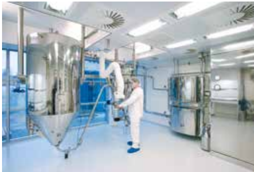
Custom-designed PHARMA-SD® type PSD-1 spray dryer in clean room.
