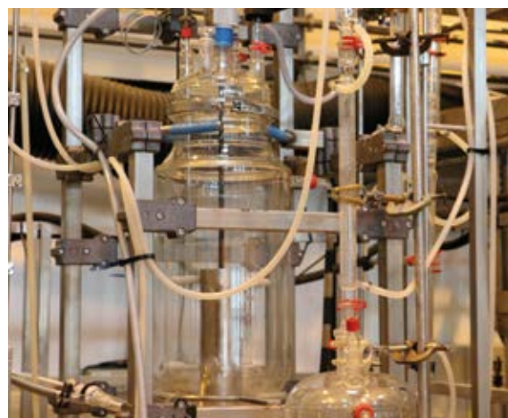
Draft Tube Crystallizer with feed and discharge tank
