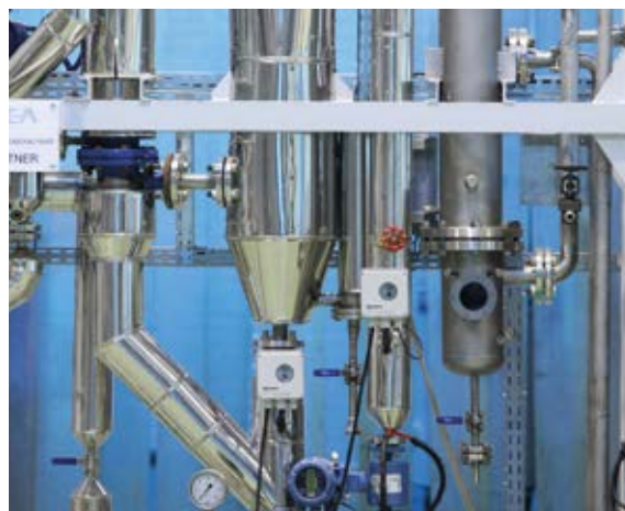
Mobile stainless steel falling film evaporator
