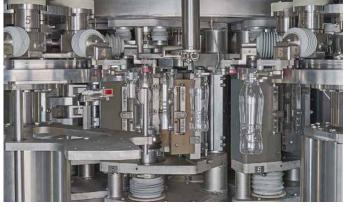
Aseptic blow molder. The sterilized preforms are blown with sterile air in an aseptic environment.
