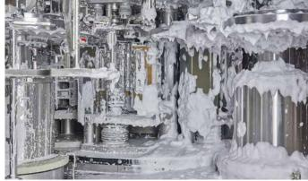
**Microbiological isolator.** With the ABF technology the aseptic stretch blow molder is located within the microbiological isolator.
