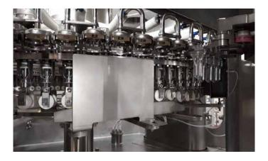
**Preform VHP treatment.** The VHP treated preforms are transferred from the sterilizing wheel to the Aseptic Blow Molder.
