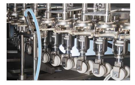
The environmental cleaning and sterilization processes are completely automated and effectively repeatable over time: they are performed via a control panel without any manual manipulation from operators that might be a potential risk of re-contamination.
