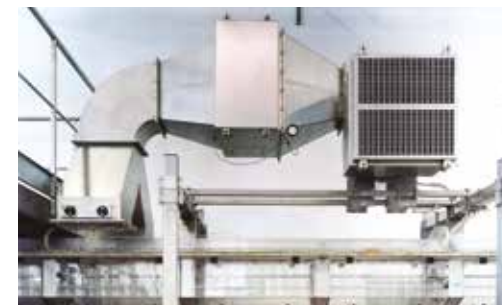
Convair air conveyor in aseptic configuration
