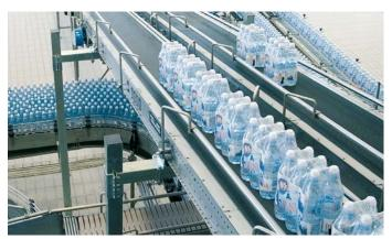
Optimized transfer solutions for "difficult" shrink wraps include rubber belt elevators/lowerators.
