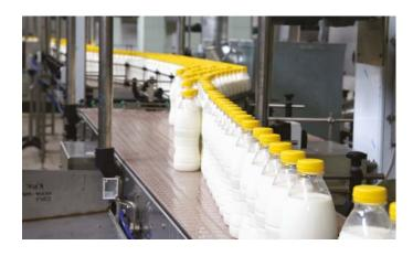
Based on production/package requirements, the conveyor design can include bottle aligners/dividers and dynamic accumulation tables.
